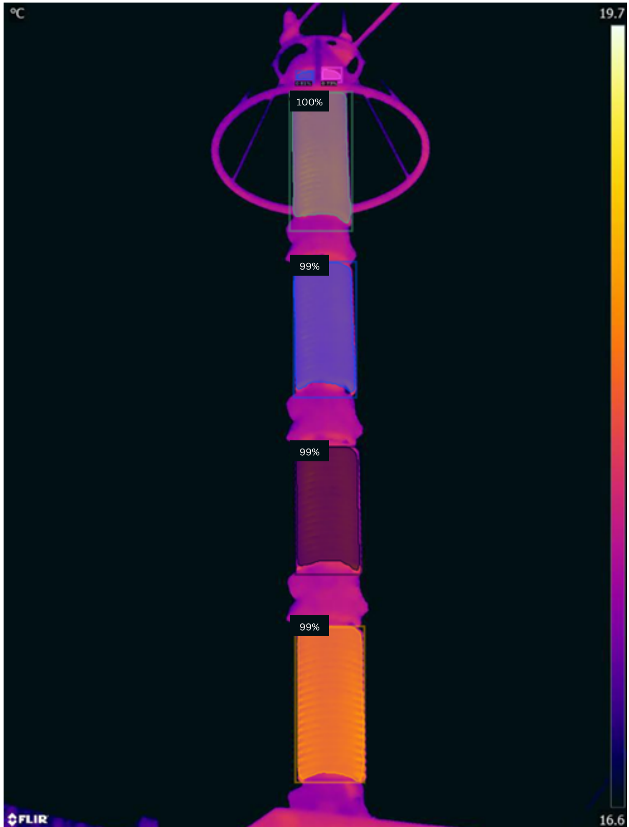
Figure 13 – Lightning arresters inference by the trained model on a test image.
