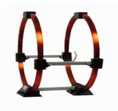
Figura 3: Bobina de Helmholtz. Fuente: PHYWE Systeme GMBH. Operating instructions. Gottingen Narrow-beam tube Pair of Helmholtz coils, Robert-Bosch-Breit 10. D-37079. 4 p.
