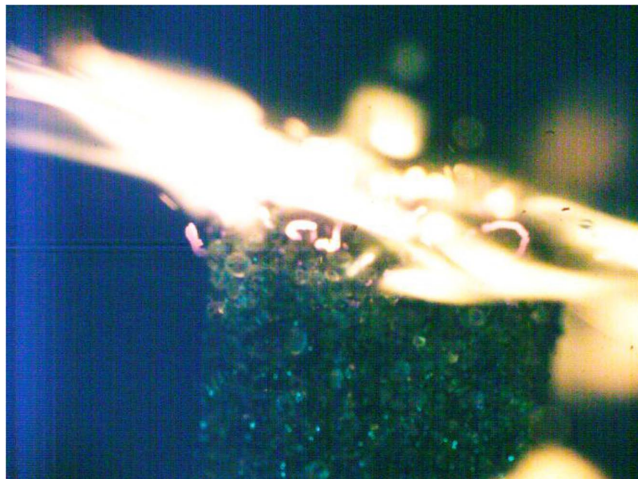
Fig. 16 Quenching process of AP-polyester propellant containing 3% EG type 1 (smallest flakes, 100 \mu\text{m} ). Actual picture width is 12.5 mm.
