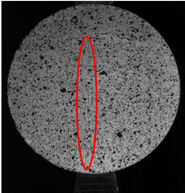
Figure 2. 12 - Sample submitted at a Brazilian test - crack initiation – diameter 40 mm – BDT15 sample
